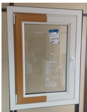
Figure 4- bio-based polyurethane window prototype
