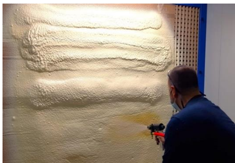
Figure 3- Bio-based PUR formulation spraying
