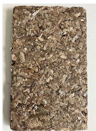
Figure 4 - Insulations from Posidonia Oceanica fibres (Photo Fraunhofer ICT, (left) NeptuTherm (right))
