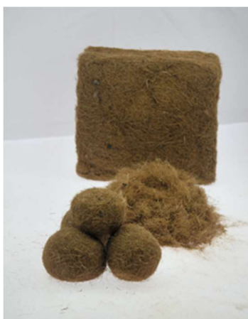
Figure 4 - Insulations from Posidonia Oceanica fibres (Photo Fraunhofer ICT, (left) NeptuTherm (right))
