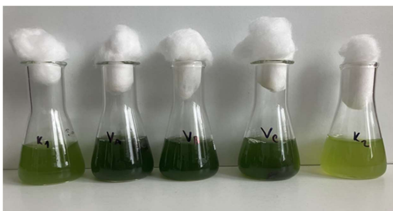
Figure 1 - Result of ecotoxicity test of Posidonia Oceanica boards to algae (samples K1 and K2 are reference samples, Va, Vb and Vc are samples with ground board particles)
