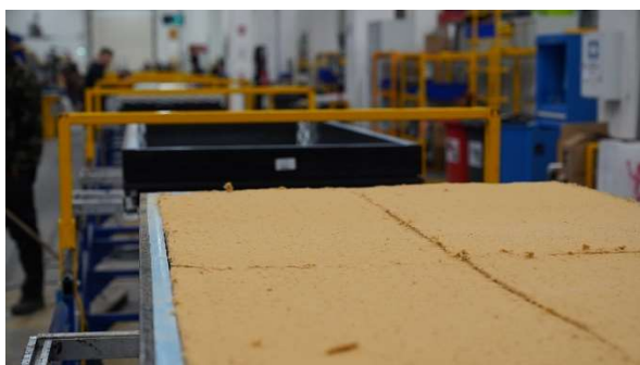
Figure 11 – Example of manufacturing process – biobased insulation assembly
