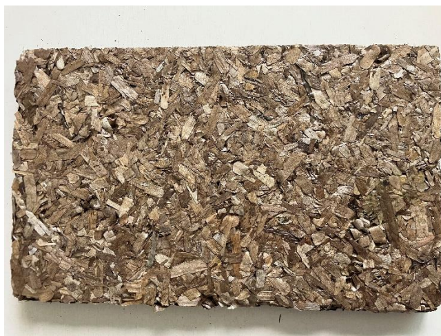
Figure 25- Particleboard from Posidonia leaves
