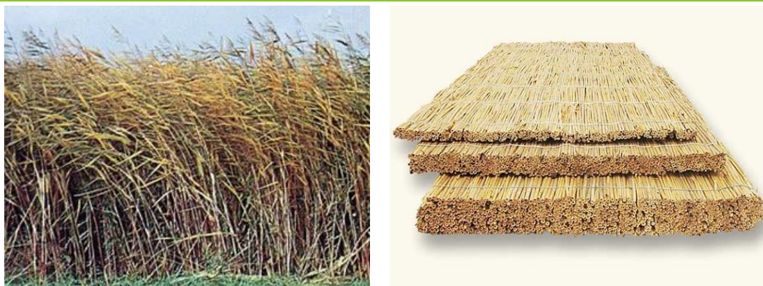
Figure 13 - Reed plant (left) and reed panel (right) (retrieved from https://www.britannica.com/plant/reed-plant and https://www.hiss-reet.de/en/building-material/reed-panel )
