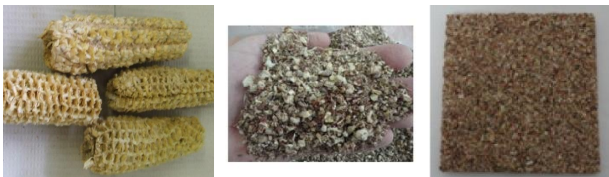
Figure 15 - Corn cobs (left). Corn cob particles (middle) and corn cob particleboard (retrieved from Paiva, 2012 )
