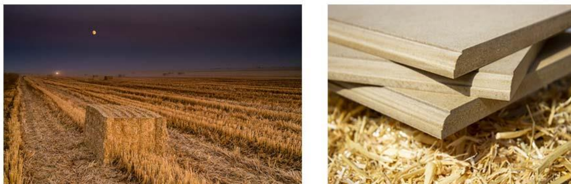
Figure 17 - Rice cropping (left) and commercial rice-straw MDF board (right) (retrieved from Beamon, 2023)
